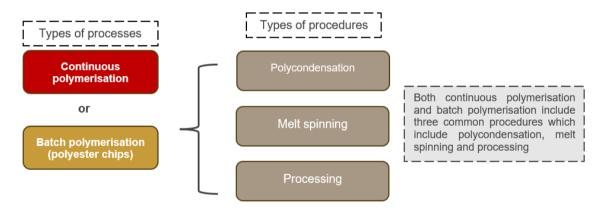
During polycondensation, the raw materials (DMT / PTA and MEG) are polymerised into polyethylene terephthalate (PET) chips. In the melt spinning stage, the melt obtained from polycondensation is converted into filament. In the third stage, the filament goes through processing activities such as drawing, crimping, heat setting, cutting, and baling.
