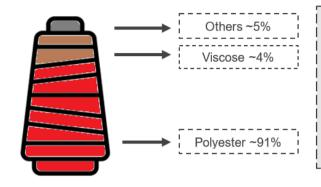
Polyester belongs to a class of polymers that primarily contain polyethylene terephthalate (PET). It is a man-made fiber which is produced using purified terephthalic acid (PTA) and mono-ethylene glycol (MEG). The two main components of the domestic MMF industry are polyester and viscose, which together account for about 95% (in volume terms). Herein, polyester accounts for about 91%, while viscose accounts for ~4%.
