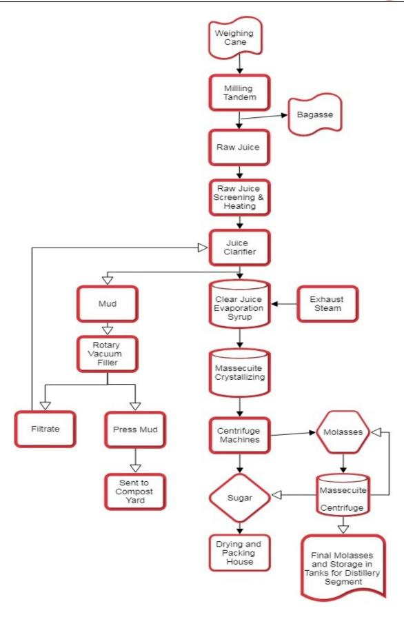
The output from the above process is then inserted in the Multiple Effect Evaporation System which results in Syrup like substance and stored in Syrup supply tanks. The Syrup in the Syrup supply tank is then subjected to the process of Crystallizing and Massecuite in various centrifuge machines giving us sugar crystals.
