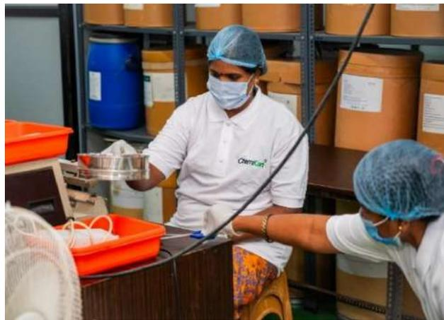
*Seaving of raw material particles taking place through seaving machine*
