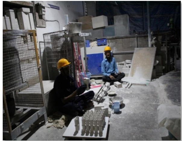
Slipcasting area-ferrule making- slip casting method is pouring of the raw material into moulds for making tubes such as ferrule
