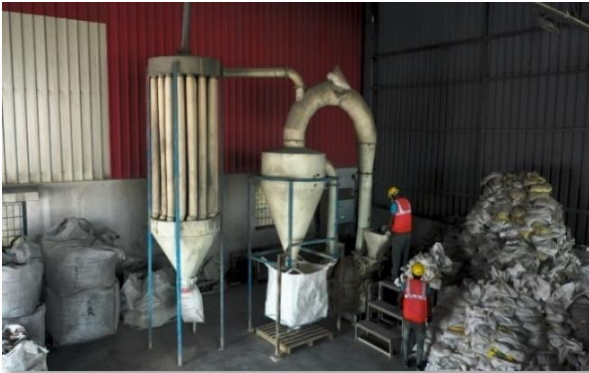
Pulverizer machine for crushing the raw material into fine powder
