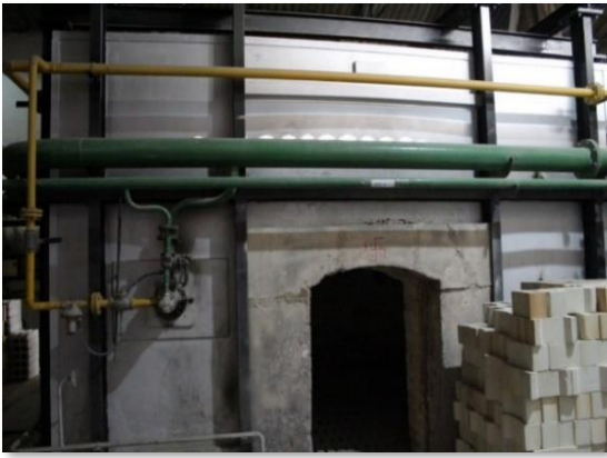
Kiln -B (10ton)- natural gas fired downdraft kiln for firing the material
