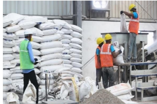
Loading the raw material into the castable machine
