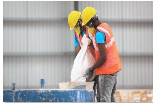
Loading of the raw material into the mixing machine
