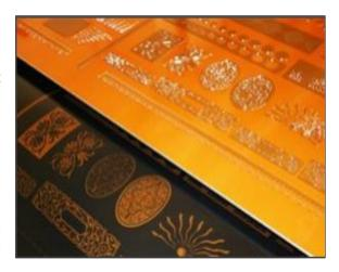
Flexographic coating plates are essential for adding protective or decorative finishes to printed materials, enhancing their appearance and durability. These finishes can provide qualities such as gloss, matte, or special effects, making them crucial in industries like label printing, packaging, and commercial printing where aesthetics and functionality are important
