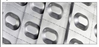
High Barrier OPA / Foil / Barrier PVC Layer is high barrier multilayer cold-formable film, it has excellent barrier against water vapor, gases and light as compare to regular. We customized the high barrier Alu-Alu foil products as per the needs of the clients.
