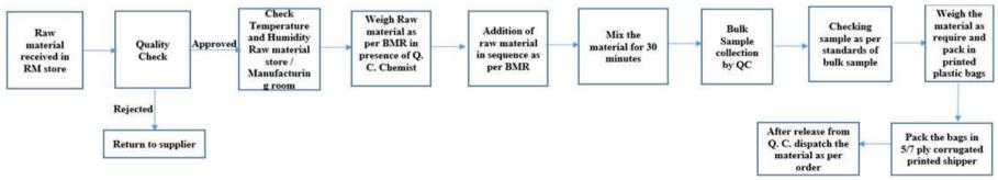
The process of manufacturing dialysis solution in Powder form is as per Indian Pharmacopia. The said Product consist of mixture of Sodium Chloride salt and Sodium biacarb salt. The salts are put in a blender and mixed thoroughly and the said mixture is the packed in aluminum pouches and used in the hospitals.
