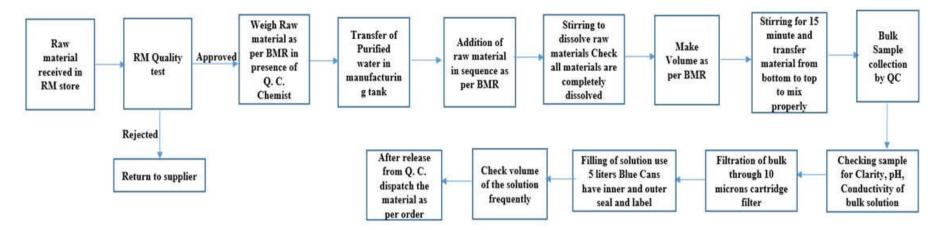
Hot Disinfectant is a Citric acid mixed with purified water, in an Stainless Steel manufacturing tank stirred and packed in a plastic can and is marketed as a disinfectant for cleaning Hemodialysis Machine
