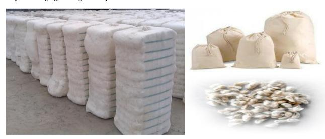
After pressing process, cotton bales are covered by protective cloth and stored on platform for dispatch. Cotton seeds are sold loosely to customers and sometimes packed in HDPE bags.
