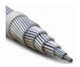
Designed to offer unique optimal strength for line design, these overhead transmission cables meet international standards including ASTM, BS, DIN, IEC, NFC etc. These are concentrically stranded conductor with one or more layers of hard drawn Aluminium wire on galvanized steel wire core which are coated with zinc with Class A Coating. The core can be single wire or stranded depending on the size of the conductors.
