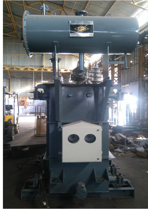
EHV Transformer of 5 mVA Capacity
