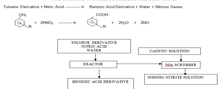
Toluene derivative corresponding to the Benzoic acid derivative to be manufactured is reacted with dilute nitric acid at high temperatures and under high pressure. During the reaction, the gases generated are scrubbed in alkali scrubber and Sodium Nitrite solution is obtained and sold. After the reaction is over the reaction mass is centrifuged, washed with water, dried, pulverised and packed. The liquid coming out of centrifuge is sent to ETP for further treatment and discharge.
