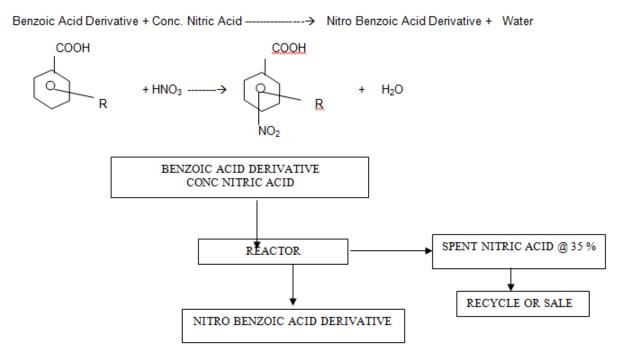
Benzoic acid derivative corresponding to the nitro benzoic acid derivative to be manufactured is reacted with concentrated nitric acid (CNA) at low temperatures. After the reaction is over the reaction mass is centrifuged, washed with water, dried, pulverised and packed. The liquid coming out of centrifuge is sent to ETP for further treatment and discharge.
